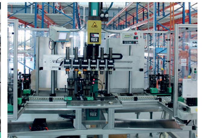
>> Press-in system for ball joint and rubber bearing
