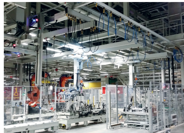
>> Handling station for front and rear axles
