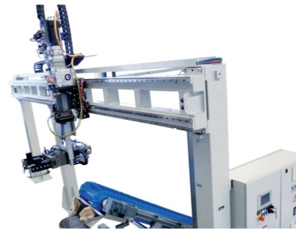
>> Track / camber adjusting machine (inlet side) with protective enclosure, operating units, workpiece carrier and position monitoring, workpiece carrier with rear axle in the station
