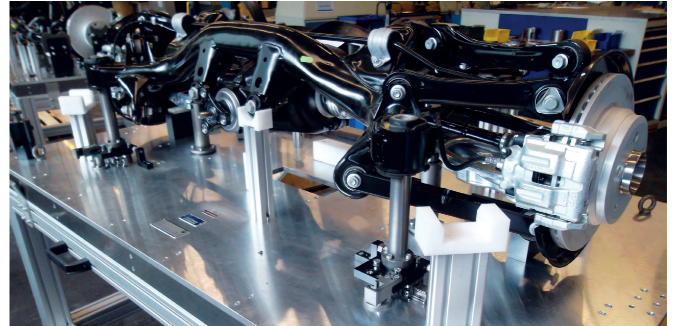
>> Front and rear axle workpiece carrier
