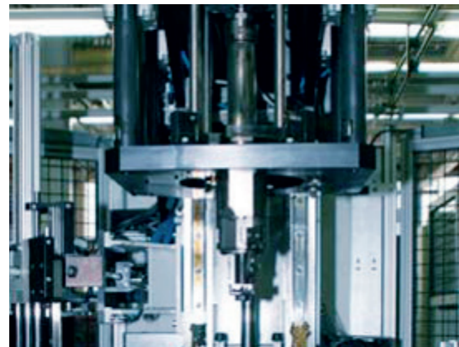
>> Wheel bearing and driver flange assembly fixture
