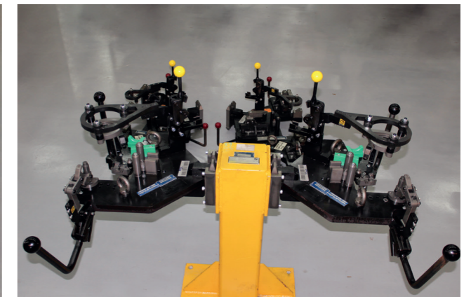
>> Wheel bearing workpiece carrier
