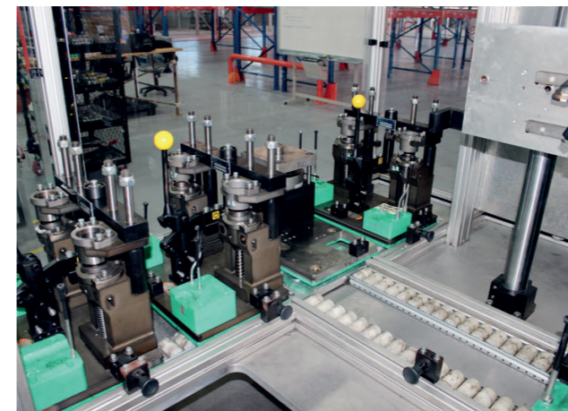
>> Wheel bearing workpiece carrier
