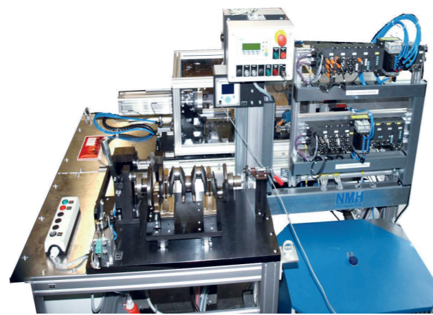
>> Station 2 (rear side): torque testing – gearwheel seat strength on crankshaft
