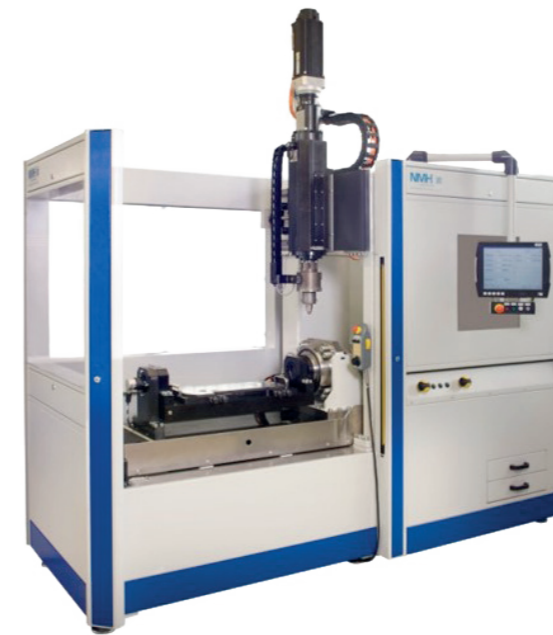
>> General view of universal assembly device for valve seat rings, valve guides and cylinder sleeves
