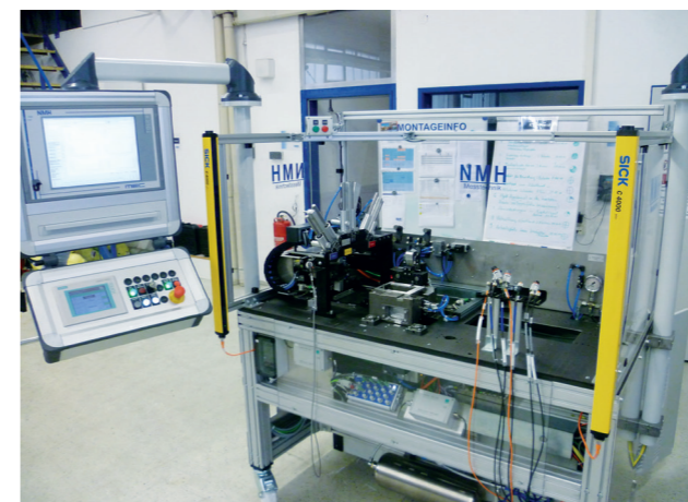
>> Test stand for shift turrets
