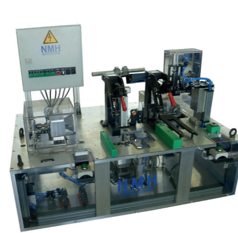
>> Calibrating dimensional control device for exhaust gas heat exchangers
