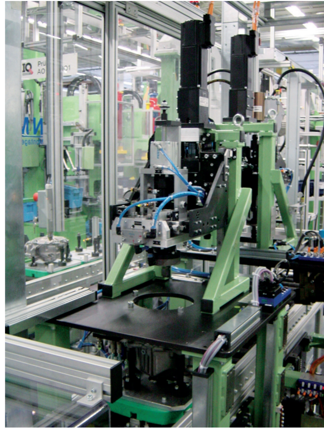
>> Front axle transmission leak test
