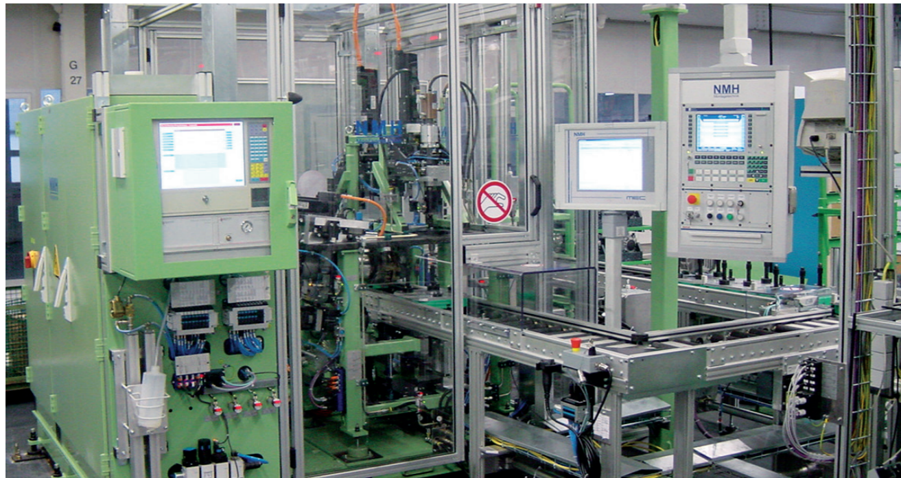
>> Overview: front axle transmission test station for tooth clearance and leak integrity
