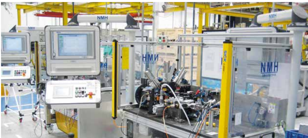
>> Measuring system for testing of shift turrets for commercial vehicle applications
