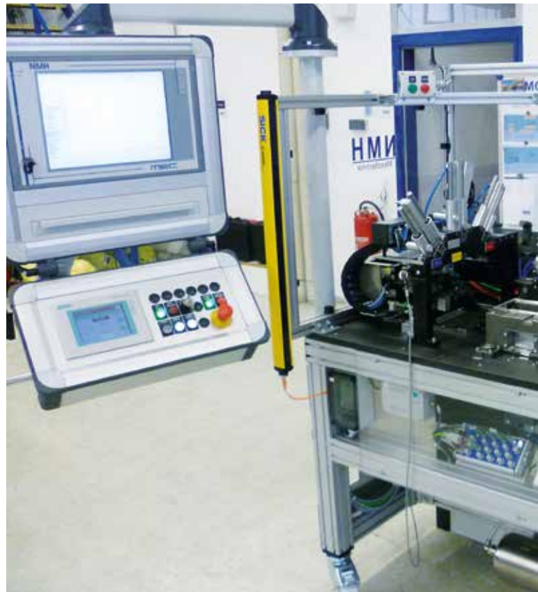
>> Measuring system for testing of shift turrets for commercial vehicle applications
